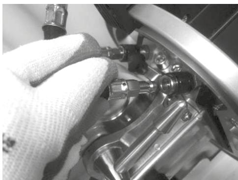
Disconnect the cooling liquid hose connector on the side of the arm tightening lever. Connect the hose connector of the draining kit instead.
