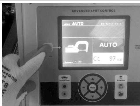
Press again the « ESC » key on the keypad to come back to the welding mode.
