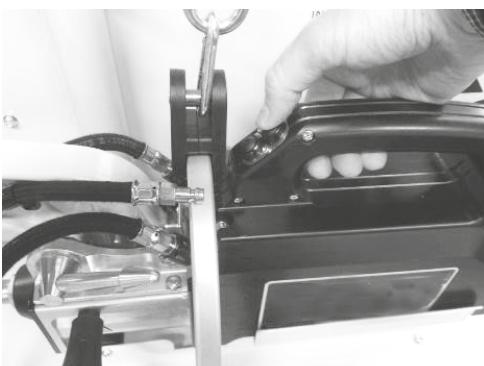
Press the top button on the clamp to activate the pump. The cooling liquid will pour out during 2 minutes, then the pump will stop automatically. When the pump stops, press again this button to continue emptying the cooling liquid tank. 20 to 30 minutes are necessary to completely empty the 30 litres inside the tank.
