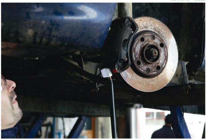
YS, the best-known manufacturer of car body repair equipment and battery chargers, has developed a range of powerful induction heaters. For decades, getting metal to expand has been done using a flame torch. Not anymore. Induction is the revolutionary method of heating metal by using electromagnetic fields. Heating from the inside out, this flameless process is much quicker, safer, and more precise than naked flame.
