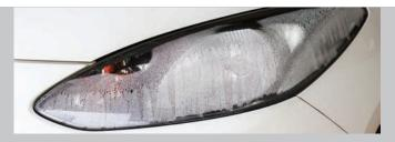
After Unprecedented Wet Weather, OEM Headlamp Manufacturer HELLA Believes Drivers Need Reminding That Fogging Or Condensation Inside Lighting Units Doesn't Usually Mean The Lamp Is Defective.
